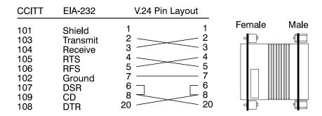
Figure B-4. Pin Assignment: RS-232 Interposer
